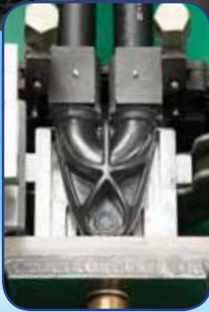
Centennial Bullet™ U-Bend fittings are fused to the Cenfuse pipe prior to shipping.
